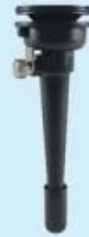
SKC GS-1 Cyclone Cat. No. 225-105 2 L/min for 4 \mu m 50% cut-point 3 L/min for 3.5- \mu m cut-point 1.7 or 2 L/min with DPM cassette
